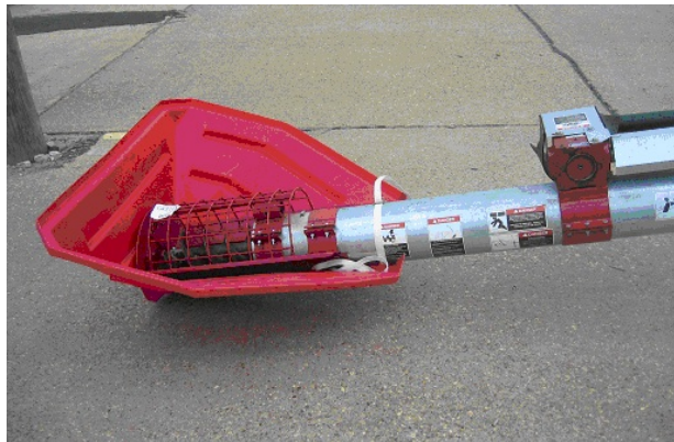
Auger with Proper Shielding and Safety Decals
